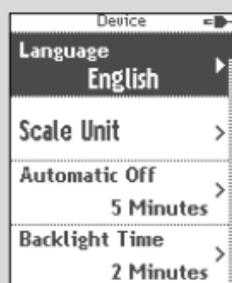
A continually visible navigation level makes the ROX GPS 7.0 menu navigation far easier for the user. The possible functions of the **BACK** and **ENTER** buttons are displayed in this level to:
